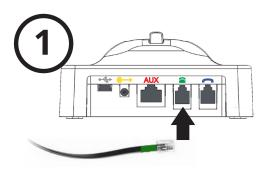
Plug one end of the telephone cord (green cord) into the Telephone Connector Port (TEL Port) on the LH270 or LH275 base
