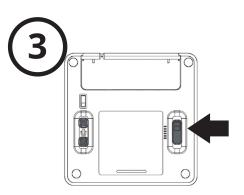
Ensure the Compatibility Switch is set correctly (most phones use setting 1). You can always call us to get the correct setting for your phone
