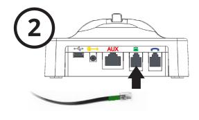
Plug one end of the telephone cord (green cord) into the Handset Jack of your phone. Plug the other end into the Telephone Connector Port (TEL Port) on the LH270 or LH275 base
