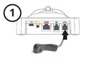
Unplug the telephone handset's curly cord from your phone base and plug into the Handset Port on the LH270 or LH275
